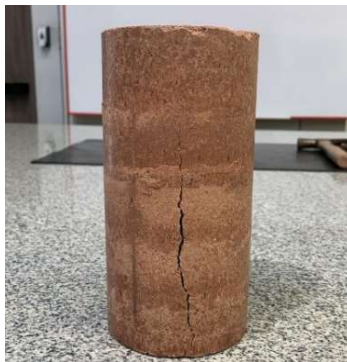
Figure 7: Cracks and fissures with mixture 2.
