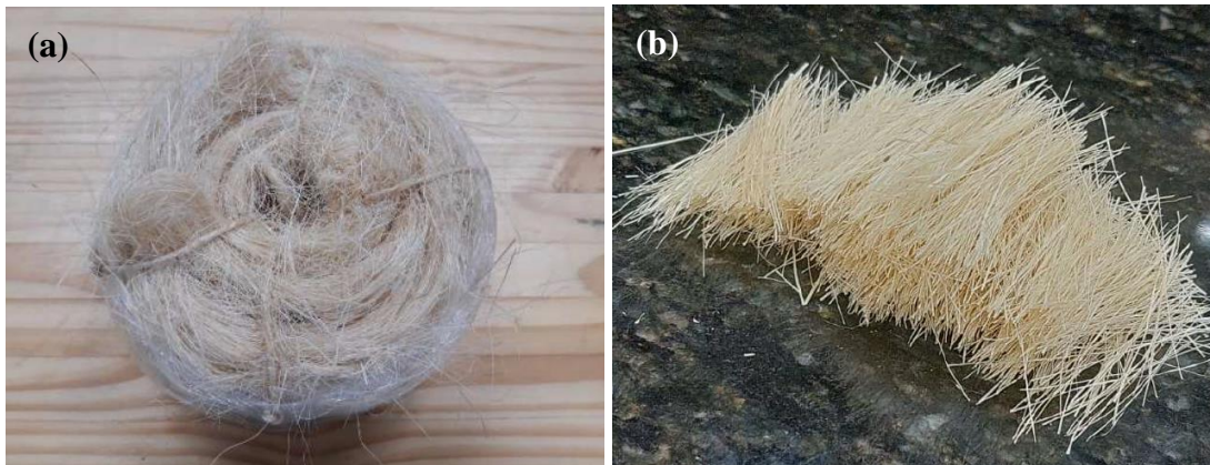
Figure 3. Natural sisal fibers: (a) Visual appearance of commercially available fibers; and (b) Fibers after preparation for testing.
